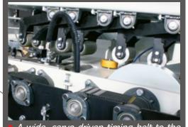
A wide, servo-driven timing belt to the bottom rollers ensures accurate cutting. This heavy-duty design has proven to be extremely durable, requiring only a minimum of maintenance.
