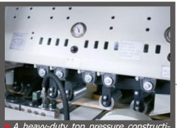
A heavy-duty top pressure construction with strong double side supported top pressure rollers. These ensure maximum contact between the workpiece and the feed roller. This enables a very reliable cut precision at a high rate of acceleration and deceleration.
