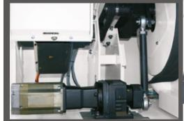
Saw blade stroke is carried out by a cam and servo motor which provide a controlable high perfomance and quality cutting at all times.
