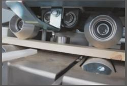
Integrated double top and bottom rollers ensure an accurate infeed of workpieces.
