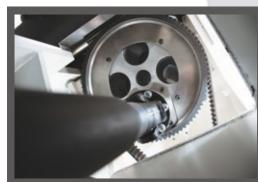
The blade stroke is characterized by a circular movement which ensures a very smooth cut with minimum tear-outs at exceedingly high cut speed.
