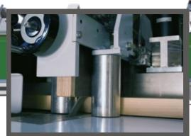
Heavy-duty top pressure unit and intelligent side rollers gives an exact cut and positioning of the workpieces during cross-cutting.
