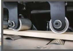
The bottom feed rollers are placed high above the bed plate of the machine. This enables the processing of bend or twisted timber, and results in maximum productivity and cut accuracy.
