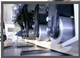
The bottom feed rollers are placed high above the bed plate of the machine which allows feeding of bend or twisted timber, ensuring maximum productivity and accuracy.
