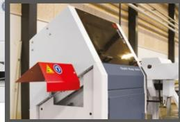
The 30° angle design of the saw secure correct workpiece positioning during cross-cutting, natural gravity for simple removal of waste and defect pieces, and easy infeed of workpieces.
