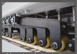
A heavy-duty infeed construction consisting of 9 driven bottom rollers and 9 top rollers. The rollers are supported on both sides to maximize the surface contact of each workpiece to provide excellent cut precision.
