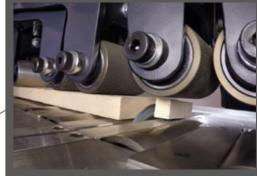
Maintenance-free mechanical waste gate ensures optimal and simple removal of small waste and defect pieces inside the saw unit, guaranteeing exact sorting of the workpieces.
