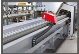
The push arm is controlled by a servo driven linear module for high capacity and cut accuracy with a minimum of maintenance.
