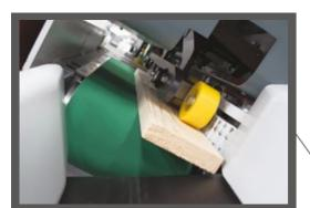
Integrated acceleration belt with driven fence for a quick and exact positioning of workpieces that exit the saw.
