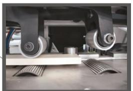
Intelligent positioning of the top rollers for fast reaction time and optimal work-piece contact. This results in a very high cut accuracy.
