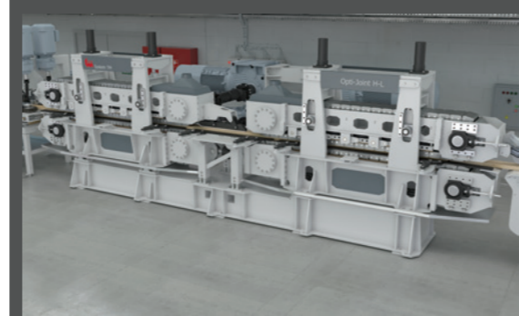
▶ Continuous press with continuous speed of last bottom and top caterpillar chain, torque controlled first bottom and top caterpillar chains for exact press force required per workpiece joint.
