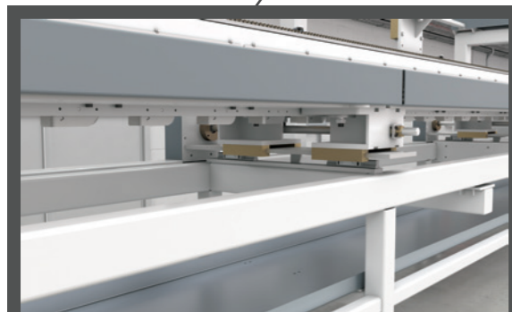
▶ Alignment station including driven side chains, one fixed and one flexible, and a driven top chain for optimal workpiece alignment before jointing of workpieces.
