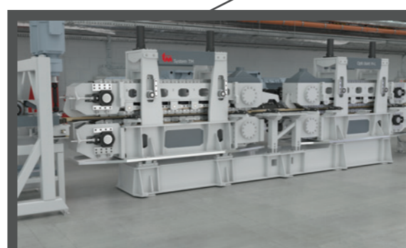
▶ Water cooling system for cooling the two upper caterpillar chains. Exhaust system to remove heat and provide ventilation from all four chains.
