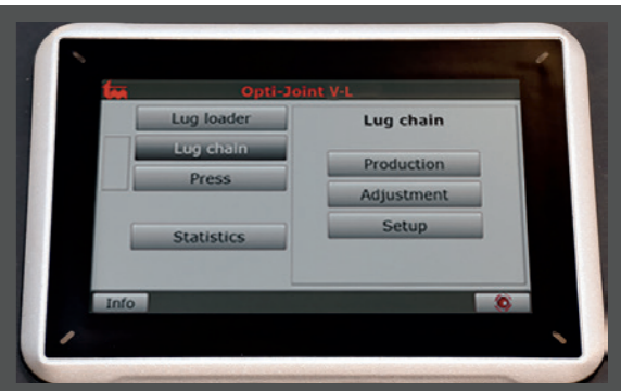
► Touch screen operator panel displaying a wide range of machine and production statistics, and quick alarm overview. Fast, easy and accurate production changeover between fixed parameter sets for each workpiece dimension.
